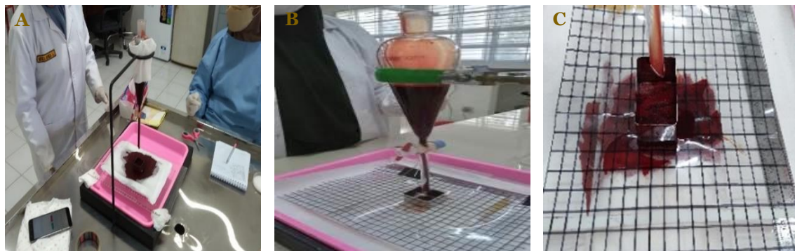
Figure 2. Experiment method for blood absorption capacity of various pads: (A) pad blood absorption capacity test; (B) blood wetted area test on the pad; and (C) measurement of blood wetted area on the pad.
